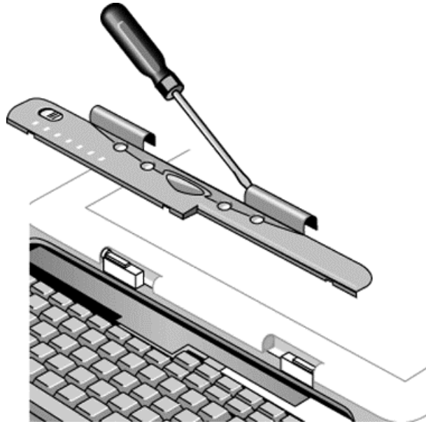
Figure 2-7. Removing the Keyboard Cover
